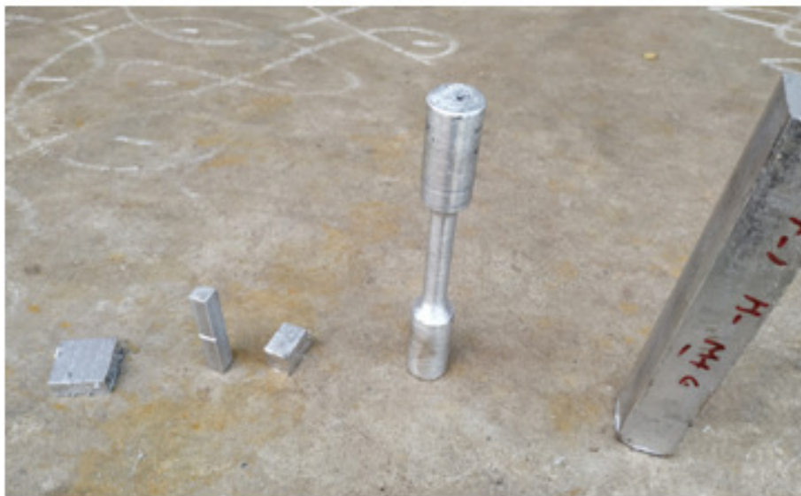
Figure 3 Tensile Test, Flexural Test, Impact Test, Hardness Test Specimens
