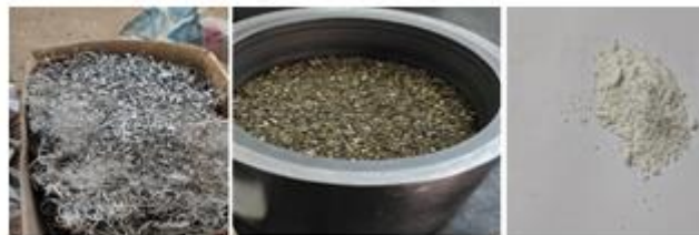
Figure 1 Raw materials of the composite material (a) aluminum scrapes (b) Vermiculite Grade v (c) Silica Powder
