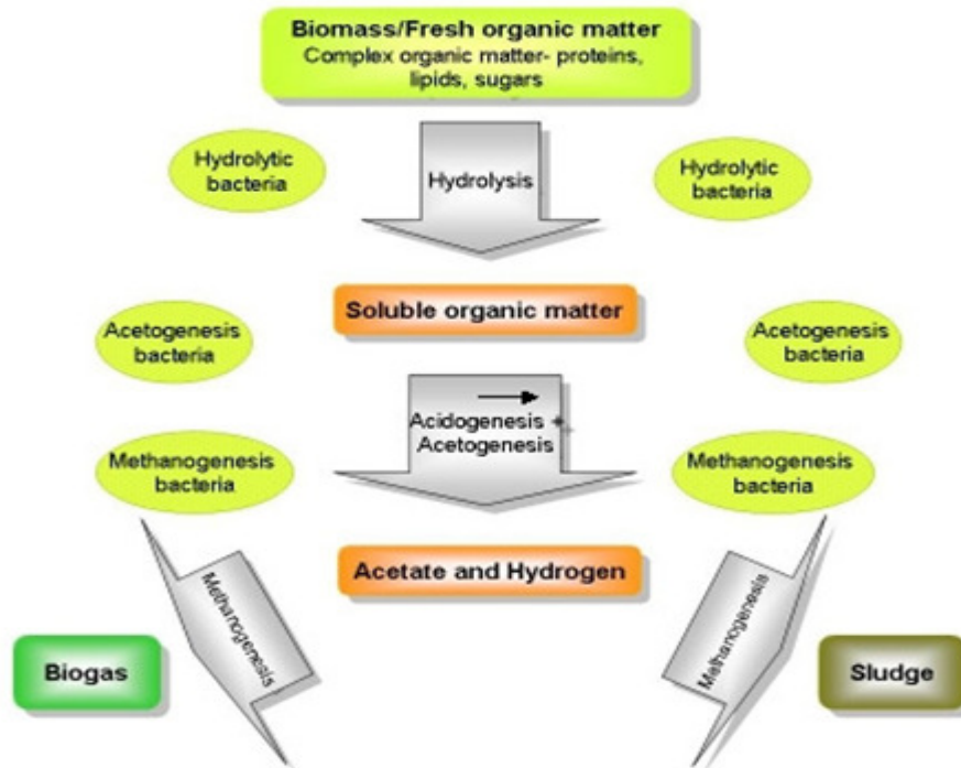
Figure 1 Stages of anaerobic digestion
