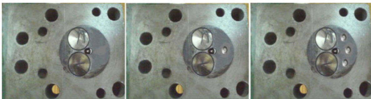
Figure 1 Normal cylinder head and Cylinder head with oval shape dimples
