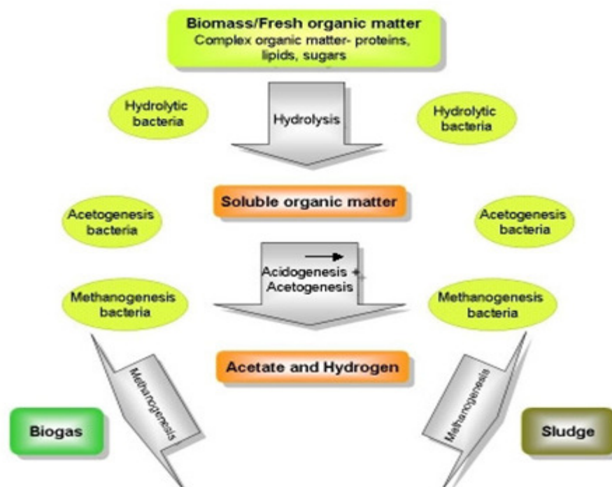
Figure 1 Stages of anaerobic digestion
