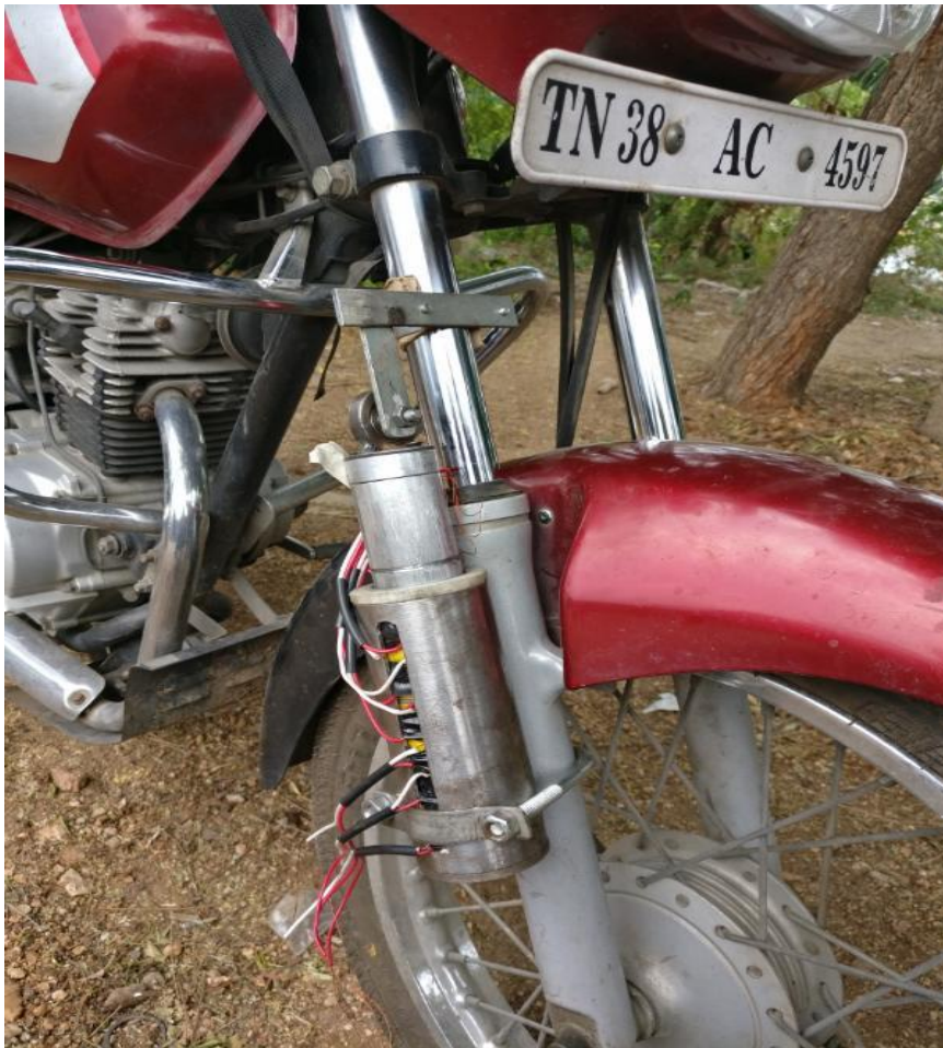
Figure 17 Shock absorber attached to the vehicle
