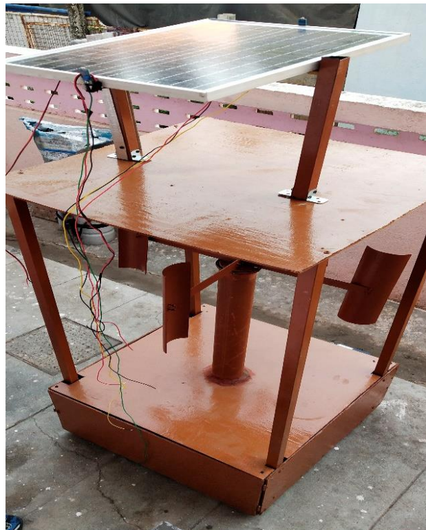
Figure 3 Fabrication Hybrid Power System
