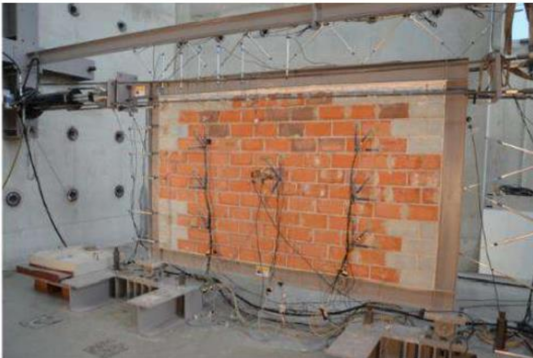
Figure. 3 SISBRICK stacked along with the conventional bricks arranged in a specific manner
