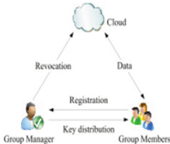
Fig.1: The system model consists of three different entities: the cloud, a manager and a large number of group members as illustrated in Fig.1.
