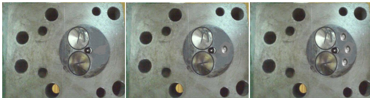
Fig 1: Normal cylinder head and Cylinder head with oval shape dimples
