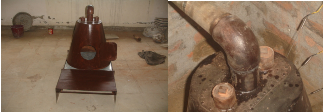
Figure1. b. Furnace of the biomass dryer with exhaust pipe.
