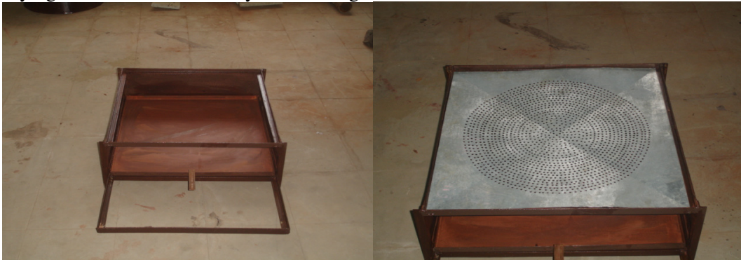
Figure1. a. Base of the biomass dryer with biomass burning tray and ash tray.
