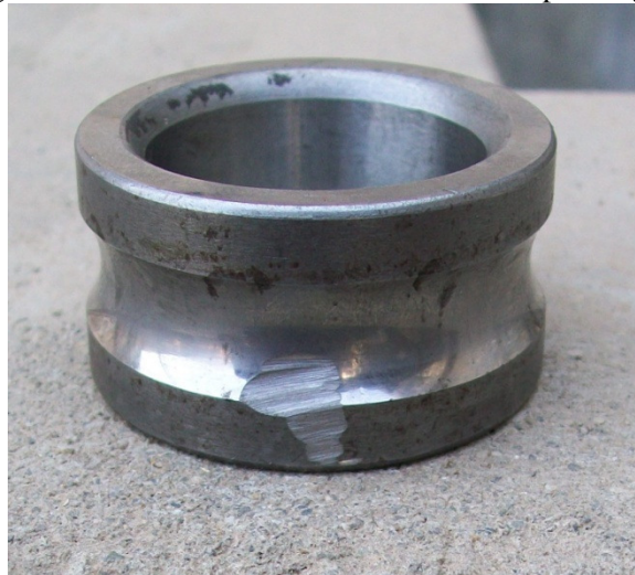
Fig 6.2: Bearing with small wear at inner race with corresponding FFT Spectrum.
