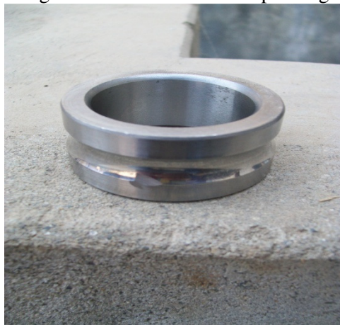
Fig 6.1(b): Bearing with no wear with corresponding FFT Spectrum
