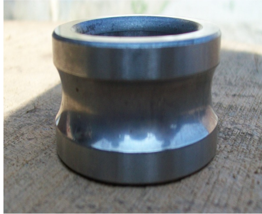
Fig 6.1(a): Bearing with no wear at inner race
